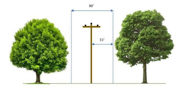
c. Minimum Line Clearance for Transmission Circuits, 69 kV:
