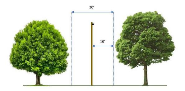
b. Minimum Line Clearance for Distribution Circuits, Three Phase:
